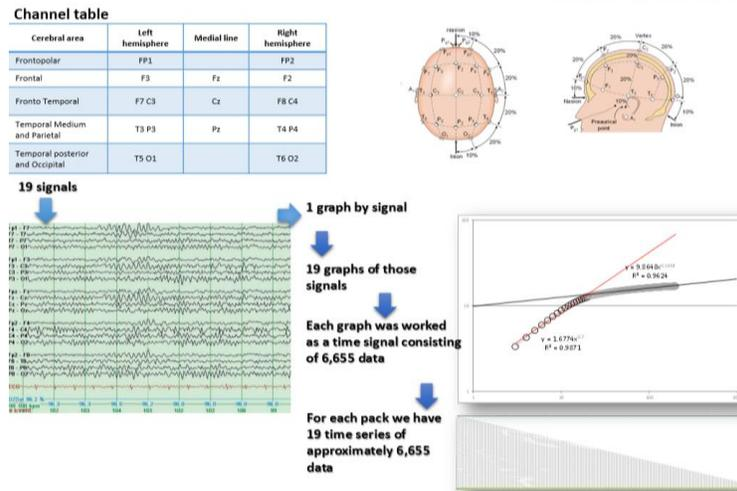
**Figure 11. EEG, signals, time series (Lina, 2018).**
