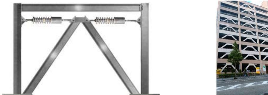
Figure-3.4 Chevron bracing with viscous damper, Chevron braced building (Yokohama)
