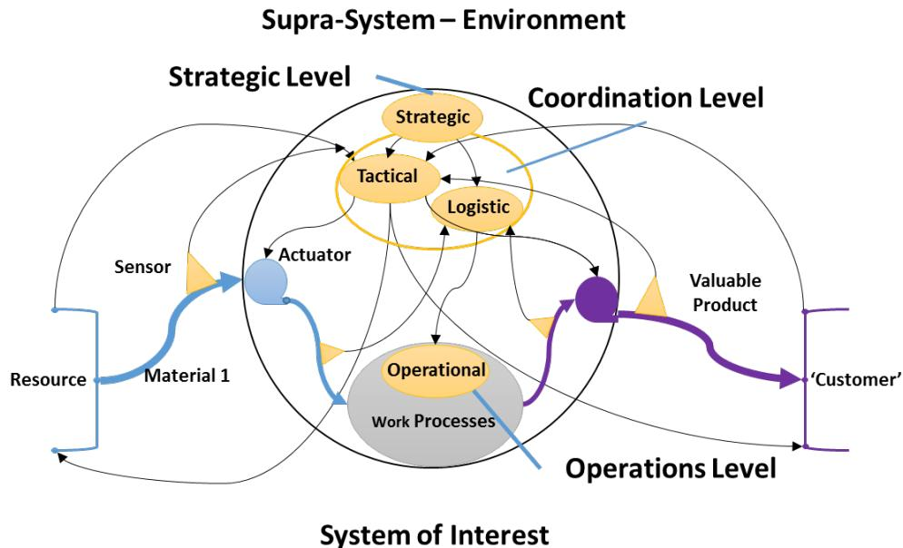
**Figure 2.** This transparent view shows the essential aspects of a purposive system with respect to the hierarchical cybernetic governance systems (yellow ovals). Yellow triangles are sensors that supply flow rate and substance quality information.
