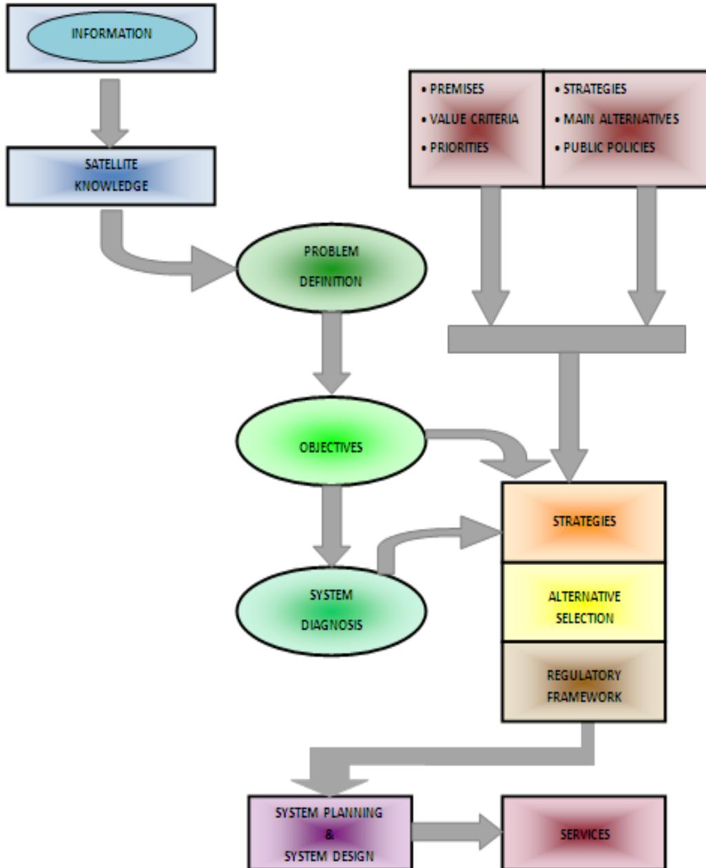
**Figure III. System Engineering Approach for Planning a New Satellite, Part I Strategies Formulation and Regulatory Framework Modification.**
