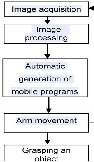
**Fig. 8 Basic Flowchart for Robot Control**
