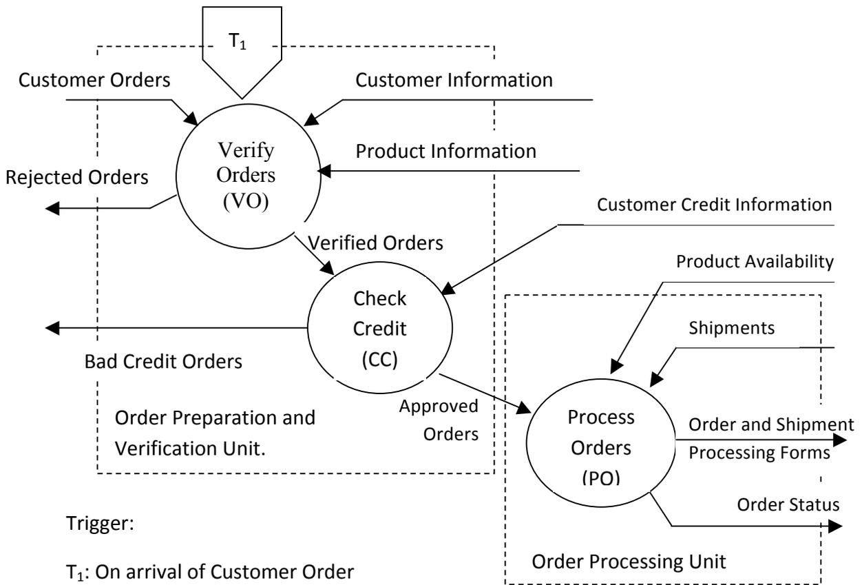
**Figure 4. Information flow diagram showing the Information processing Functions (IPFs) Verify Order (VI), Check Credit (CC), and Process Order (PO). The arrows show information flows between these IPFs and between them and the external environment.**
