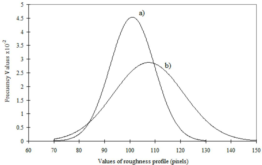
**Figure 4.** Gaussian distribution of the interfaces roughness profiles in the borided samples at temperature of 1193 K and 6 h of treatment time, with boron paste thickness of: **a)** 4 mm, **b)** 5mm.
