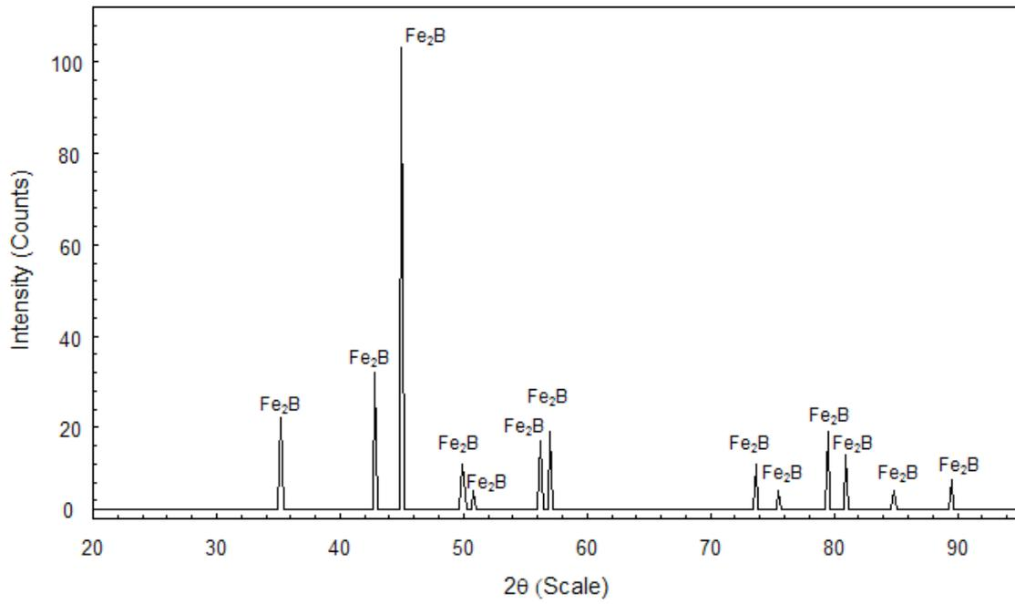
**Figure 2.** XRD pattern for AISI 1045 steel borided at 1223 K with 6 h of treatment and 5 mm of boron paste thickness.
