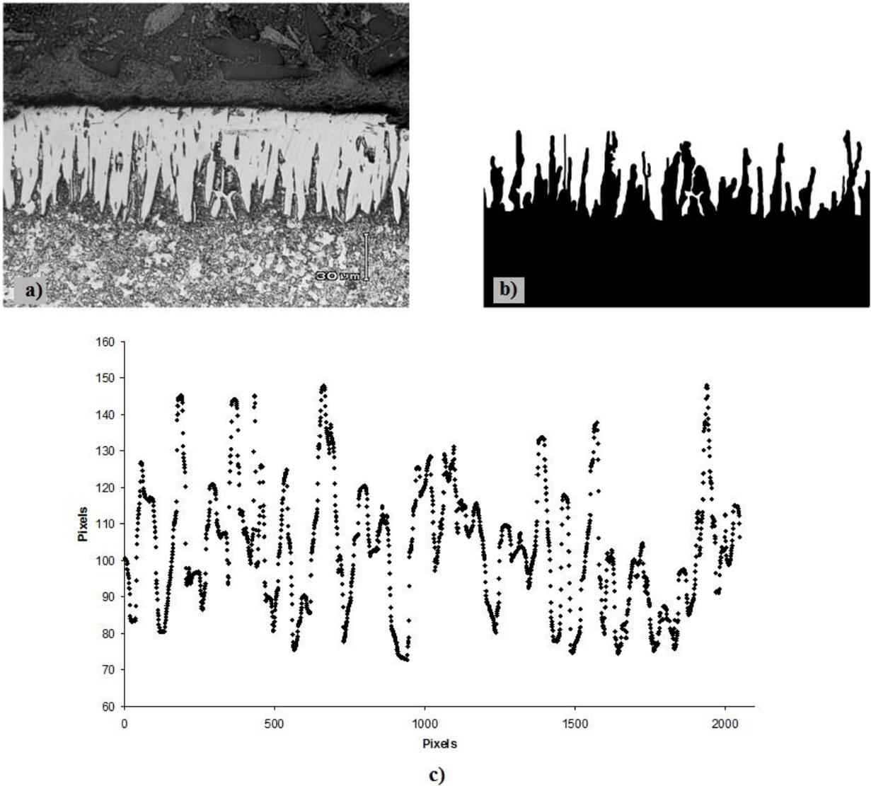
**Figure 1.** a) Cross sectional view of the borided sample at 1223 K, with exposure time of 4h and boron paste thickness of 5mm, b) the same image digitalized in binary colours c) image interpretation with aid of Scion Image Software.
