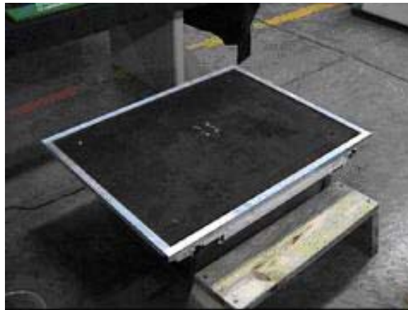
Fig 4. Simulator of earthquakes with variable intensity developed at the ESIME-Z-IPN
