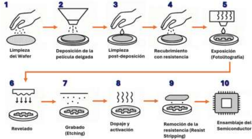
Exhibit 2. Semiconductor manufacturing process
