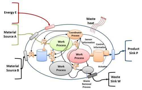
Figure 7. Deconstruction of the SOI in figure 6 (partial) shows how the lexical elements of SL are used to construct the structural description of the internals (transparent view). Note the use of interfaces receiving and emitting flows to/from the SOI. Internal energy distribution is not shown to avoid clutter, however there is a subsystem that captures and distributes energy to all of the work processes, similar to that shown in figure 1.
