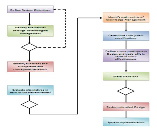
Figure IV. System Engineering Approach for Planning a New Satellite Part II Design Basis
