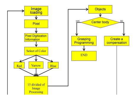
Fig. 4 Flowchart of Image Processing
