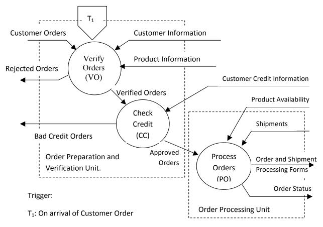
Figure 4. Information flow diagram showing the Information processing Functions (IPFs) Verify Order (VI), Check Credit (CC), and Process Order (PO). The arrows show information flows between these IPFs and between them and the external environment.
